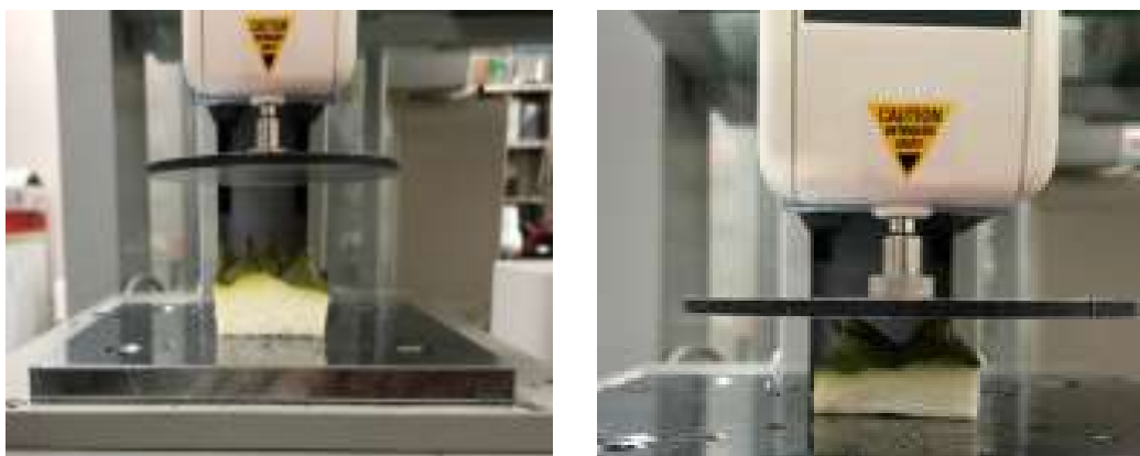
Figure 2. Compressive strength of durian peel.
