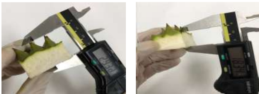
Figure 1. Thickness of fresh durian peel: (a) thickness of spiny peel; (b) thickness of non-spiny peel.
